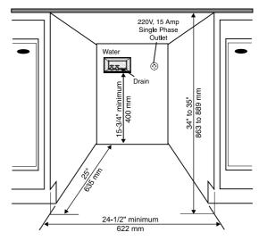
If the drain outlet is higher than 24", the connections will need to be recessed.
